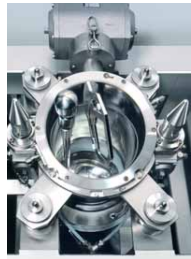
Washing station for IBCs with passive valves
