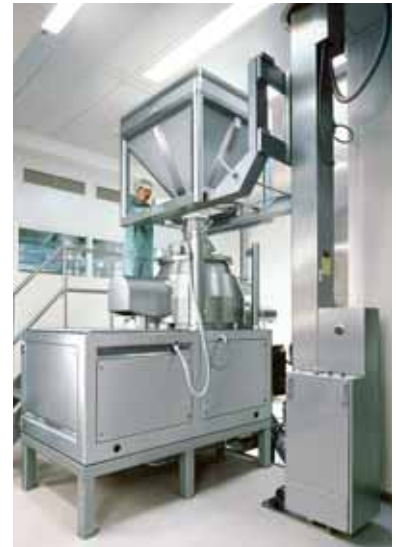
L 1500 lifting device for discharging containers into a VG 600 vertical granulator
