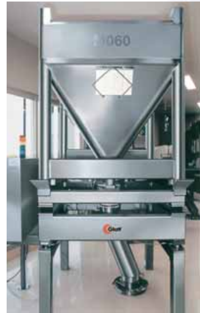
Container discharging station above a tablet press
