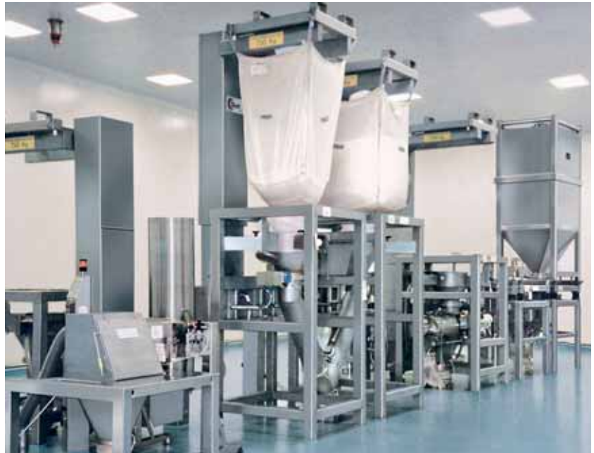
Raw material dispensing from sacks, big-bags (super sacks) and IBCs
