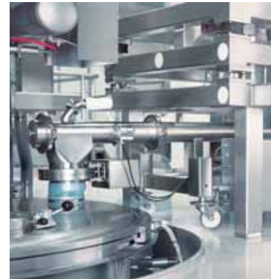
Mobile SDS feeder, docked
