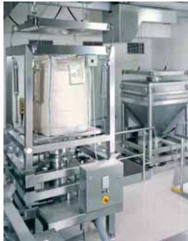
Discharging station, universal for containers and big-bags
