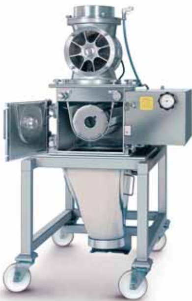
Rotary feeder, with practically no gap, for even dosing and filling
