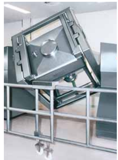
CMK 1000 special design, mixing between two columns
