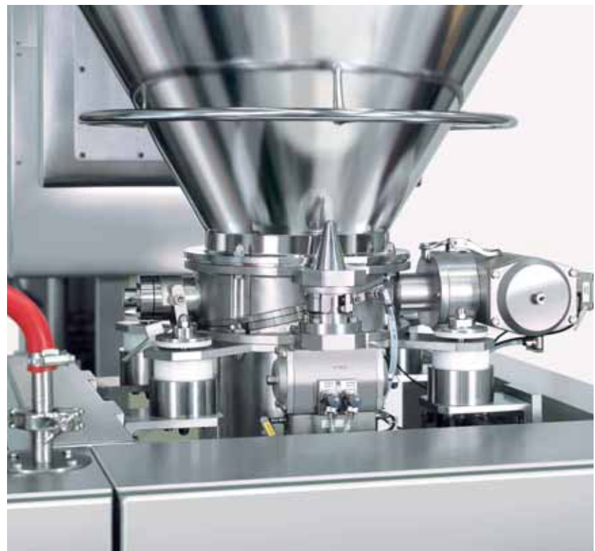
IBC discharge using the Glatt SKS isolation valve system
