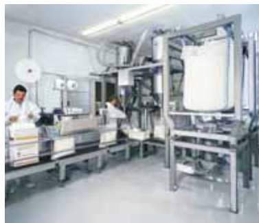
Pneumatical discharge of big bags for ready-made packaging
