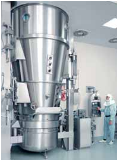
Fluid bed granulating and coating with a Glatt GPCG 300
