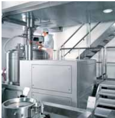
High-shear granulation with a Glatt VG 800 vertical granulator
