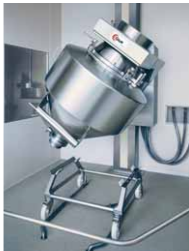
CMR 1000 container blender for round container
