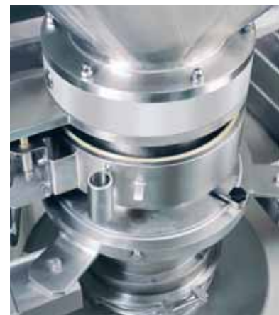
Docking system using an inflatable radial seal, after docking
